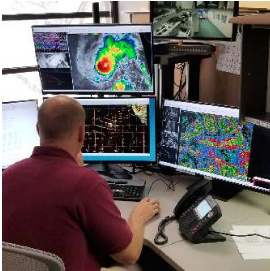
A National Weather Service (NWS) meteorologist in Honolulu, Hawaii, reviews weather data from NOAAPort in the Advanced Weather Interactive Processing System (AWIPS) while coordinating with emergency response partners via telephone in June 2018
