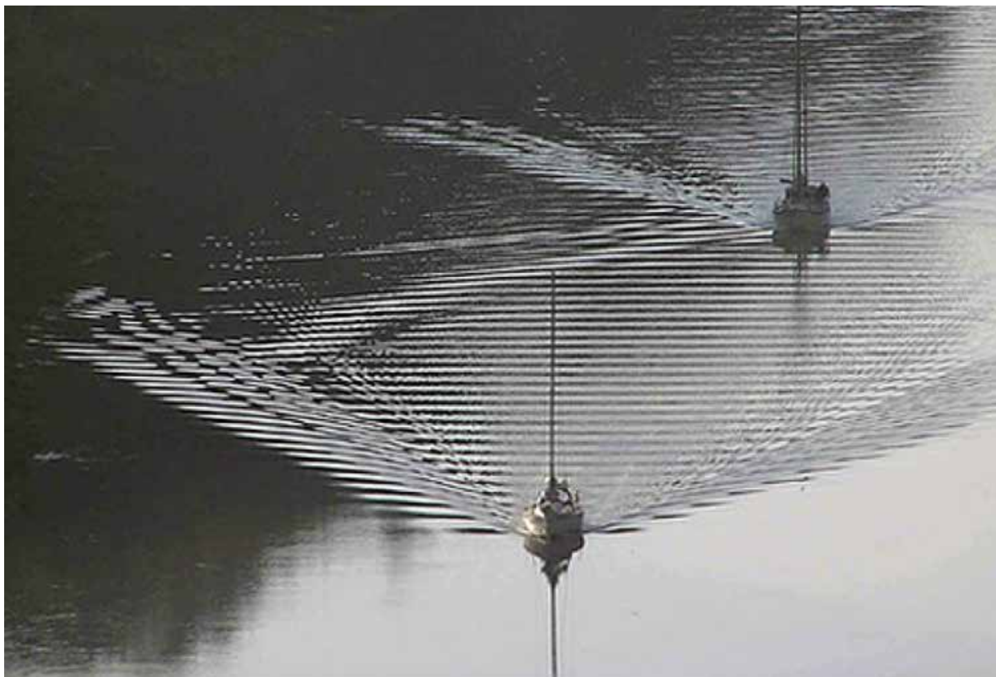
FIGURE 9-12. A boat's bow and stern waves travel out from the ship as wave trains. If you look carefully at the bow wave of the leading boat, you can see that the leading wave disappears as it moves away from where the boat has passed and is replaced by another wave behind it. The second wave in turn disappears to be replaced by another one behind it, and so on. The wave energy is also slowly spread as the wave crest lengthens by dispersion, and the wave train eventually disappears. Note how the bow and stern waves of the two boats combine to form complex wave interference patterns.
