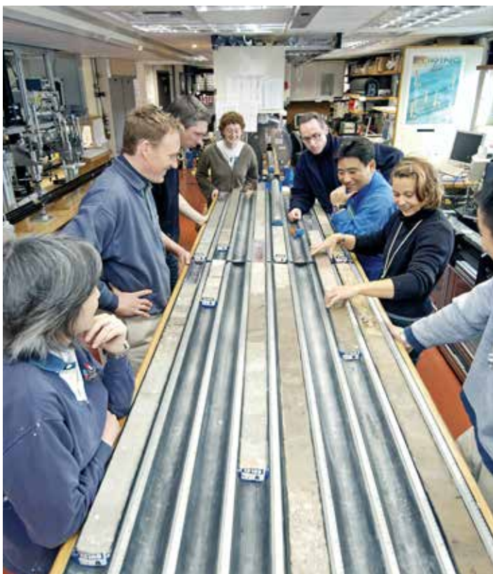
FIGURE 6-20. Sediment cores, such as this deep-sea drilling core, are first cut down the middle and then marked every 1 to 2 cm, each 1–2 cm section representing the accumulation of sediments during a period of hundreds or thousands of years in the past.
