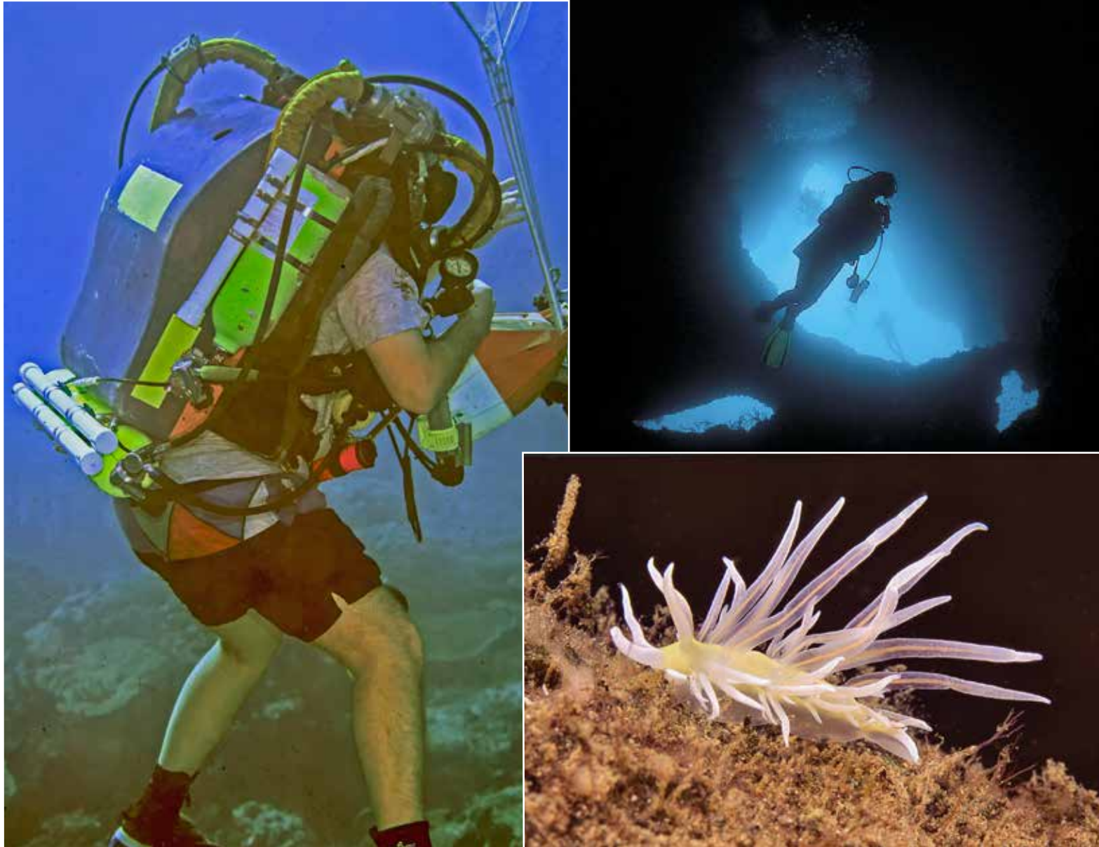
FIGURE 3-1. Developments in scuba diving technology are revolutionizing marine sciences. The strange-looking backpack on the diver shown in the image on the left is a scuba rebreather system that removes carbon dioxide that the diver breathes out so that the gases can be rebreathed many times. Rebreather systems use a computer to control the mixture of air, oxygen, and helium that the diver breathes allowing divers to make very deep dives and return to the surface safely without the many hours of decompression that are usually needed. The spectacular nudibranch shown in the photo to the right is one of many never-before-seen species found on a number of very deep dives made with the rebreather in Papua New Guinea. It was collected from a depth of about 130 m. Scuba is normally limited to a maximum depth of about 50 m.
