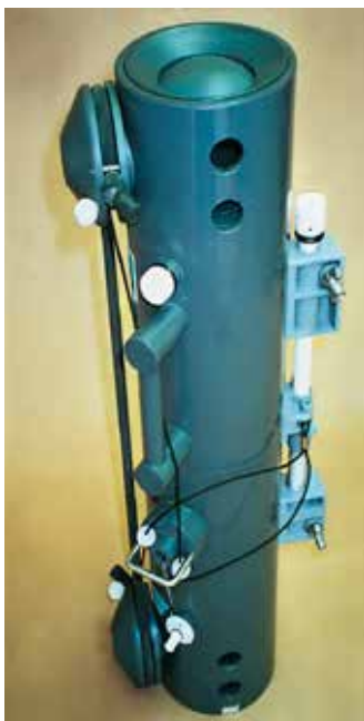
FIGURE 3-12. A Go-Flo water-sampling bottle. This ingeniously designed bottle is lowered through the sea surface in a closed configuration to avoid contamination. At a depth of a few feet, a pressure-sensitive trigger opens both ends of the bottle. The bottle is closed again by means of a messenger or other triggering device when the bottle is at the required sampling depth.
