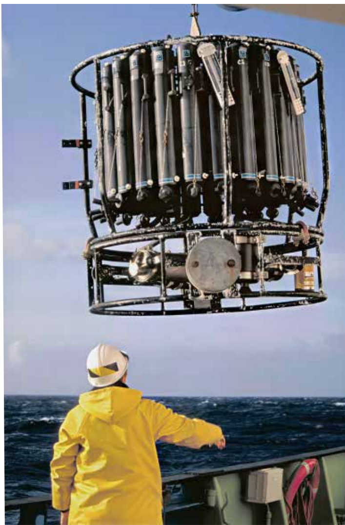
FIGURE 3-14. AA rosette water sampler has sample bottles, some fitted with thermometer racks, arranged in a rosette pattern around an electronic device that enables researchers on the ship above to close individual sample bottles at selected depths through an electrical signal sent down the hydrographic cable. The round frame below the water-sampling bottle rack usually contains a CTD and possibly other sensors, such as turbidity-measuring devices.
