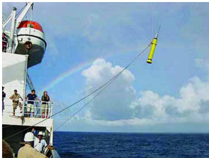
FIGURE 3-25. An Argo float system is deployed from a research vessel to begin its long unattended journey through the ocean depths.
