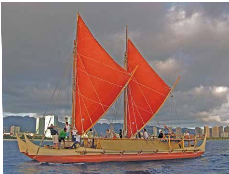
FIGURE 2-4 The Hokule'a . This vessel is a reproduction of the double-hulled voyaging canoes that the Polynesians used to explore and colonize the Pacific.
