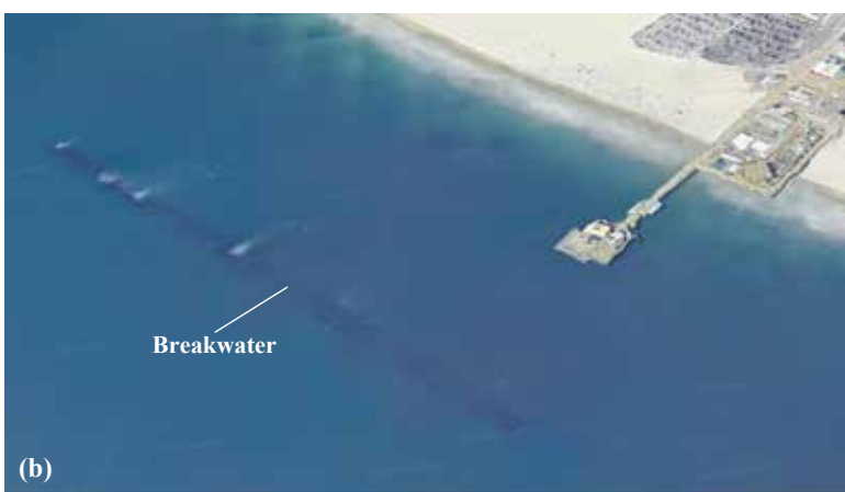
FIGURE 11-27. (a) Some boat harbors consist of a breakwater or jetty built parallel to the shore. The breakwater protects boats but also interferes with the longshore drift by blocking the waves from reaching the beach behind the breakwater. (b) In this image the submerged remains of the Santa Monica harbor wall (the dark line almost parallel to the shore) are parallel to the beach line. When it was first built, before it sank, the wall blocked enough wave energy to allow sand to build up on the beach under the pier so the harbor became too shallow and unusable. The wall has now sunk deep enough that its effect on the longshore drift is much reduced. The pier is elevated on pilings, which allows the wave energy to pass through. As a result, the pier does not block the longshore drift. (c) Offshore breakwaters are used not only to create harbors but also to control coastal erosion as in this satellite image of an area near Norfolk, Virginia. The built up spits of sand behind each of the segments of the offshore breakwater are caused by the interruption of longshore drift. This type of segmented breakwater temporarily slows overall erosion but many would consider that it also makes the beach unnatural and unsightly.
