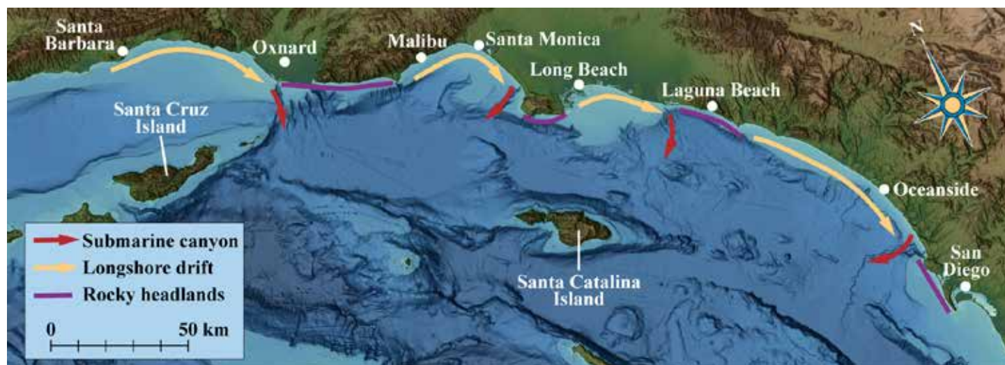
FIGURE 11-18. There are several north-to-south littoral drift cells in southern California. Each of these cells ends at the head of a submarine canyon where the sand is lost as it is transported down the canyon.
