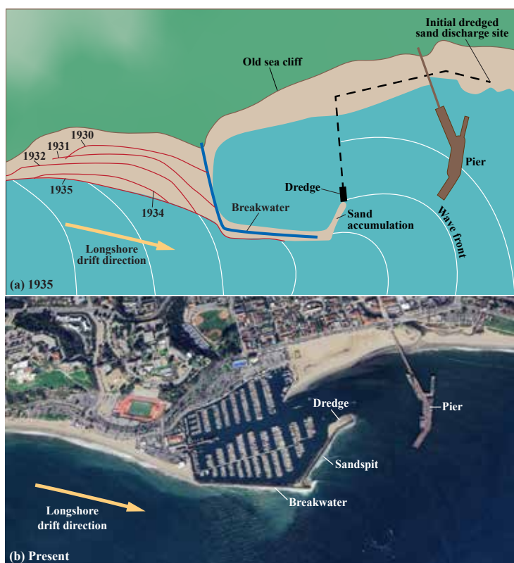
FIGURE 11-26. The jetties of the Santa Barbara harbor breakwater have interfered with the longshore drift transport system. (a) When the breakwater was first built, sand accumulated and progressively widened the beach on the north side of the main jetty (the direction from which waves most often come, the left in this photo) until the sand began to be transported south again. However, sand transported around this breakwater cannot be transported across the deep harbor mouth and accumulates in a spit inside the harbor mouth. The beach on the south side of the harbor has had its supply of sand from longshore drift cut off. Periodic but continuous dredging is needed to keep the harbor from silting up. The dredged sand is deposited on the south-side beach to prevent this beach from eroding further. (b) Since the breakwater was first constructed this satellite image shows how the deeper channel in the harbor mouth provides a break in the wave pattern that interrupts the longshore drift. The sand spit that developed has now been armoured with rocks, and dredging continues from the area at the end of the spit where sand still accumulates. This sand is still dredged annually, pumped through a pipeline, and discharged on the beach farther down the coast than the original discharge location. Note the sports stadium, roads, parking lots and other buildings now built on the area of sand accumulation on the left of the breakwater that was previously ocean where longshore drift carried sand accumulated to extend the beach within the first few years after the breakwater was built.
