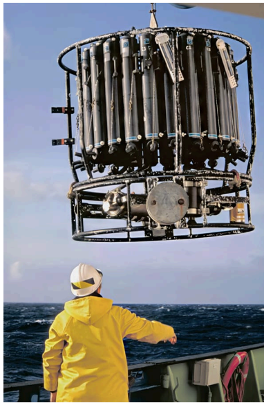
Figure 3-14. A rosette water sampler has sample bottles, some fitted with thermometer racks, arranged in a rosette pattern around an electronic device that enables researchers on the ship above to close individual sample bottles at selected depths through an electrical signal sent down the hydrographic cable. The round frame below the water-sampling bottle rack usually contains a CTD and possibly other sensors, such as turbidity-measuring devices.
