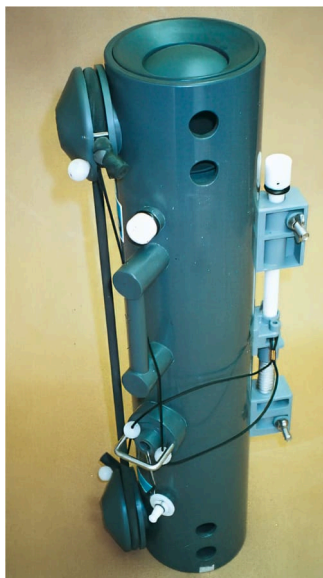
Figure 3-12. A GoFlo water-sampling bottle. This ingeniously designed bottle is lowered through the sea surface in a closed configuration to avoid contamination. At a depth of a few feet, a pressure-sensitive trigger opens both ends of the bottle. The bottle is closed again by means of a messenger or other triggering device when the bottle is at the required sampling depth.
