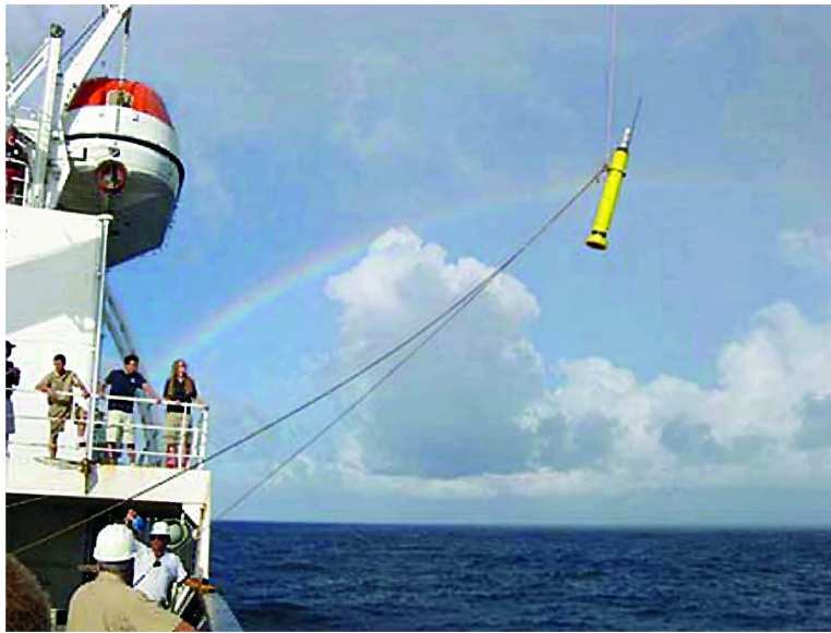
Figure 3-25. An Argo float system is deployed from a research vessel to begin its long unattended journey through the ocean depths.
