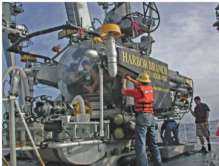
Figure 3-23. A typical submersible, such as the Johnson Sea Link shown in this photograph, consists of a glass or plastic sphere inside a hull. The scientists descend within the sphere, which is provided with air and heat. Motors, articulated arms, and many different types of samplers and cameras are mounted outside the sphere. These are used to provide propulsion and collect samples.
