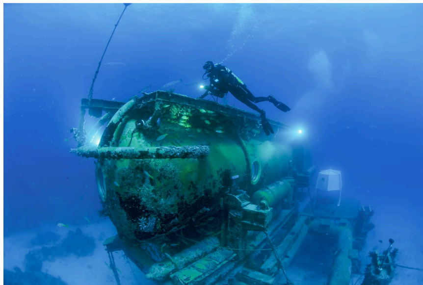
Figure 3-22. Underwater habitats, such as Aquarius, shown here in the Florida Keys, enable scientists to live and work up to several tens of meters underwater for several days without incurring decompression sickness. However, at the end of their stay they must undergo very long decompression periods in a decompression chamber.
