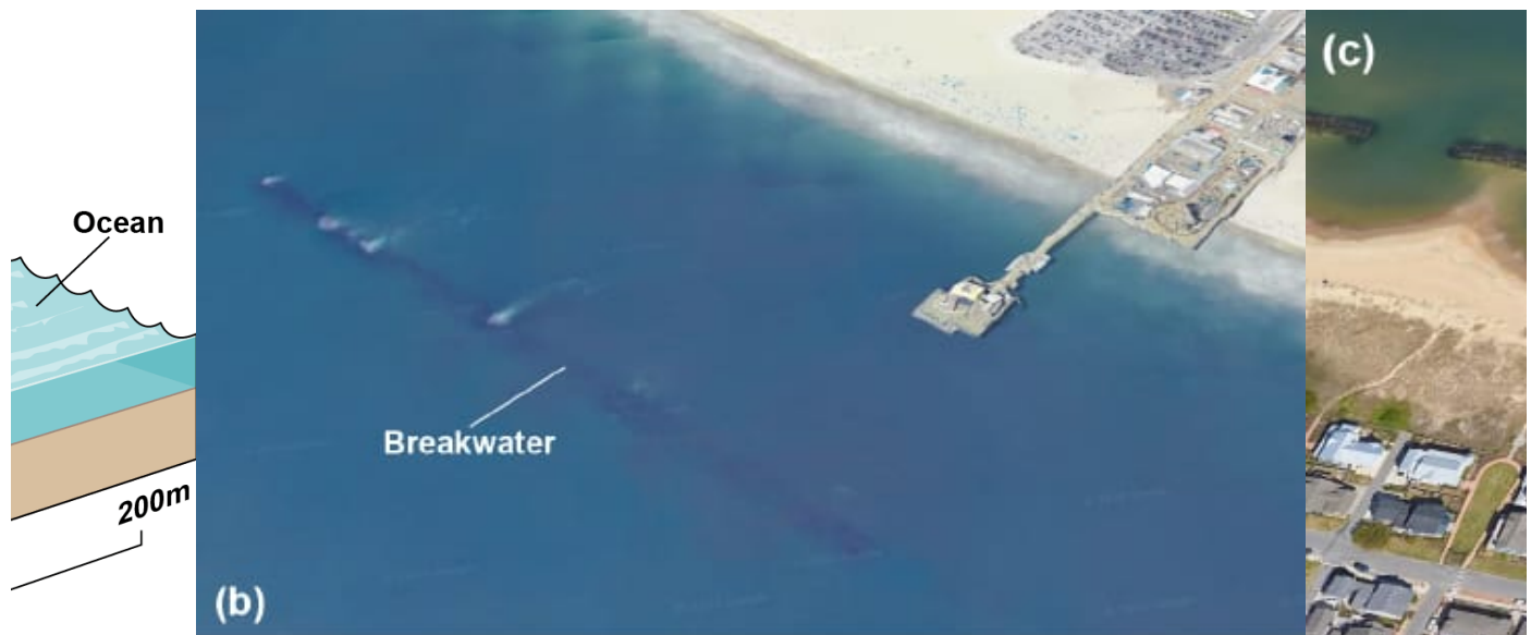
Figure 11-27. (a) Some boat harbors consist of a breakwater or jetty built parallel to the shore. The breakwater protects boats but also interferes with the longshore drift by blocking the waves from reaching the beach behind the breakwater. (b) In this image the submerged remains of the Santa Monica harbor wall (the dark line almost parallel to the shore) are parallel to the beach line. When it was first built, before it sank, the wall blocked enough wave energy to allow sand to build up on the beach under the pier so the harbor became too shallow and unusable. The wall has now sunk deep enough that its effect on the longshore drift is much reduced. The pier is elevated on pilings, which allows the wave energy to pass through. As a result, the pier does not block the longshore drift. (c) Offshore breakwaters are used not only to create harbors but also to control coastal erosion as in this satellite image of an area near Norfolk, Virginia. The built up spits of sand behind each of the segments of the offshore breakwater are caused by the interruption of longshore drift. This type of segmented breakwater temporarily slows overall erosion but many would consider that it also makes the beach unnatural and unsightly.
