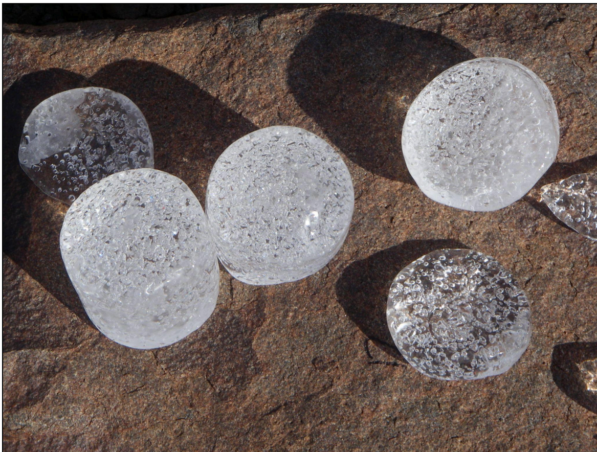
Figure 11. An ice core can reveal a great deal about the prior climate. The bubbles in ice are trapped atmospheric gases that will be sent to various laboratories for analysis. These samples are from Beacon Valley, Dry Valleys, Antarctica. [Photo by Jacquelyn Hams (PolarTREC 2008) , Courtesy of ARCUS ]
