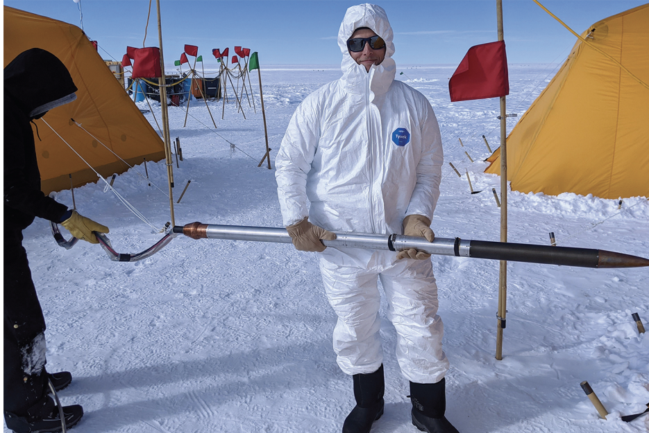
Figure 11. A scientist testing the ice diver on the Greenland ice sheet. The tip of the ice diver is metal and contains thermal wiring that melts quickly through the ice. [Photo from the University of Washington Applied Physics Laboratory]
