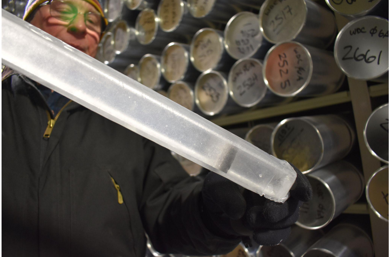
Figure 12. A scientist at the Ice Core Facility shows an ice core with a brown-gray layer of volcanic ash in it. [Photo by Kelsey Lindsey]
