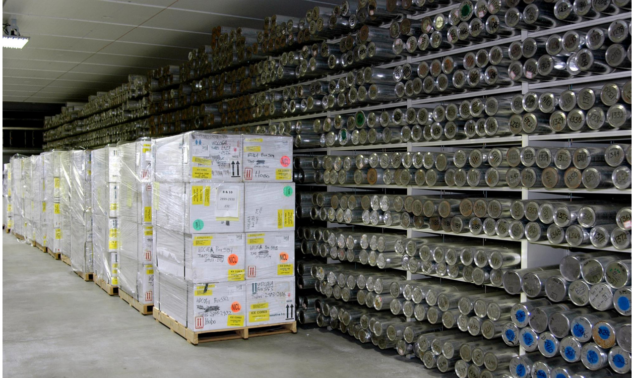
Figure 15. Silver tubes of ice stored in the freezer at the National Science Foundation Ice Core Facility in Denver, Colorado. Each tube contains 1 meter (3.28 feet) of ice and the white boxes contain recently-drilled ice from the West Antarctic Ice Sheet (WAIS). [Photo by Peter Rejcek]
