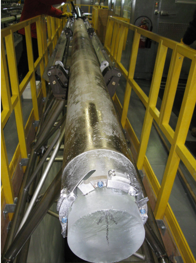
Figure 13. Recently drilled ice core sticking out of the drill sonde. Note the arrow helping the scientists to orient the core the same way it was oriented in the ice sheet. [Photo by Peter Neff]
