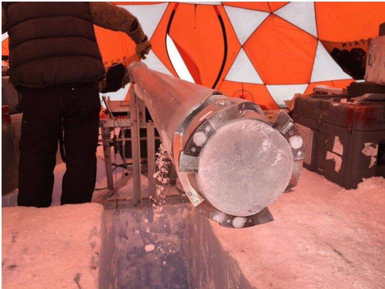
Figure 7. An ice core extracted during the 2015/16 field season at Allan Hills, Antarctica. [Photo by Yuzhen Yan]
