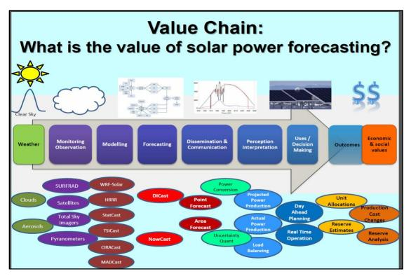
Figure 13: Solar Power Forecasting Value Chain (Source: Haupt et al. 2018)
